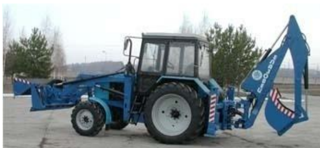
➤ Axially adjustable backhoe loader EP-2630E
